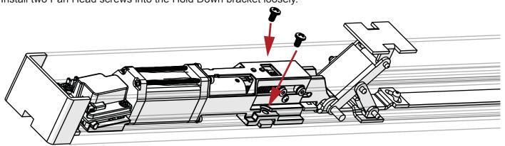
6. (1) depress and hold the activating linkage down completely, (2) push and hold the kit towards the head of the device, (3) continue to holds the kit in position while you release the activating bracket and secure the kit into position by tightening the screws on the hold down bracket.
