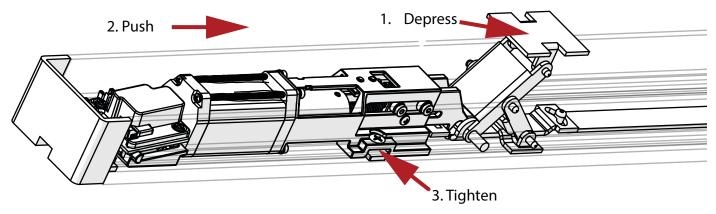
Replace push pad, test function and adjust PTS location if needed (see page 4). Once complete, install end **7**. caps to finish the installation.
