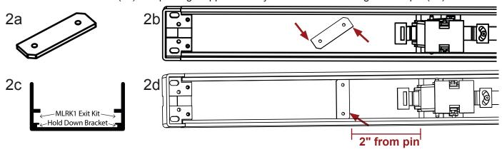
Hold motor kit perpendicular to the device placing the tail end into the housing (3a), identify the MLRK1 Exit 3. Kit channel (2c) and rotate the kit 90 degrees to lock it into the channel (3b), depress the activating bracket and allow the kit to lay over the top of the hold down bracket and activating bracket pin (3c).
